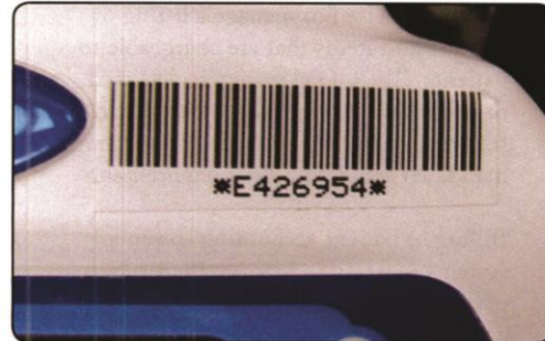
Figure 21.4 Barcode scanning systems are an example of computerized methods used to track assets, such as equipment.
